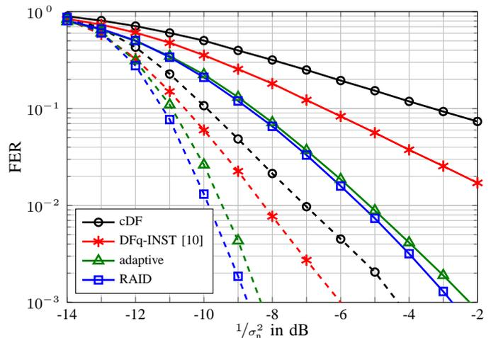
Fig. 8. FERs at the destination for common detection (cDF), modified detection with weighting from [10] (DFq-INST), the adaptive relay scheme and the proposed RAID scheme for  $L = 1$  (solid) and  $L = 4$  (dashed) channel taps.
