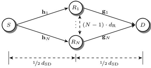
Fig. 1. Topology of the considered two-hop relay system.
