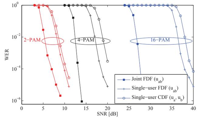
Figure 6. Word error rates for the single-carrier TWRC with fast Rayleigh fading for  $\{2, 4, 16\}$ -PAM
