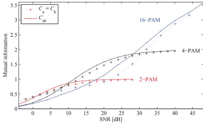
Figure 5. Mutual informations  $C_a = C_b$  for complete and  $C_{ab}$  for functional decoding
