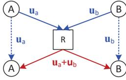
Figure 1. The two-way relay channel: Users A and B want to exchange their information packets  $\mathbf{u}_a$  and  $\mathbf{u}_b$  via the relay R. There is no direct link between the users.
