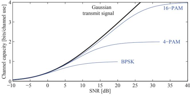
Figure 2. Channel capacities for fast Rayleigh fading
