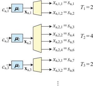
Figure 4. Symbol to subcarrier mapping in the uplink of the multi-carrier two-way relay channel
