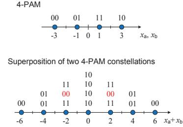
Figure 3. Superposition of two 4-PAM constellations. The bit labels for the combined symbols  $c_{ab}$  are not unique for some constellation points.
