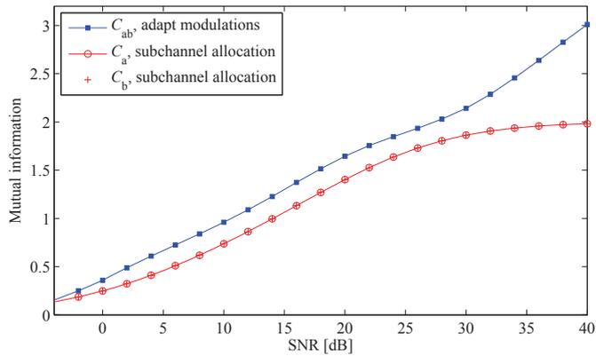
Figure 7. Achieved mutual informations with subchannel allocation for complete decoding and rate adaptation for functional decode
