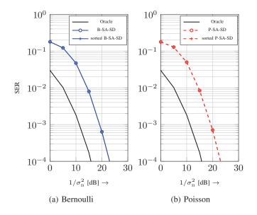
Figure 5: a), SER results for B-SA-SD with or without sorting; b) SER results for P-SA-SD with or without sorting.
