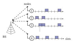
Figure 1: Sporadic uplink transmission of multiple devices communicating with a BS. Each time slot corresponds to one data frame and the system is assumed to be synchronous.
