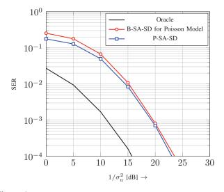
Figure 4: SER results for MAP detection given in (6) with P-SA-SD and the B-SA-SD applied for the Poisson model here for comparison.
