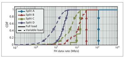
**Figure 3.** Cumulative distribution function (CDF) of required FH data rates of different functional splits considering full load in all BSs (solid lines) and considering a varying load (dashed lines).
