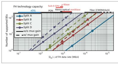
**Figure 4.** 99th percentile of the aggregated FH data rate (including safety factor) vs. the number of aggregated BSs.
