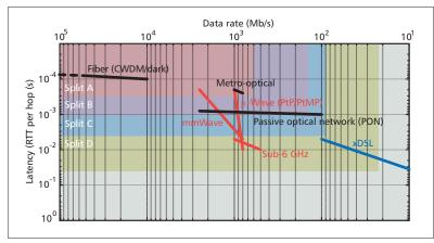
**Figure 2.** Latency and data rate requirements for different functional splits vs. available FH technologies.
