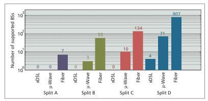
**Figure 5.** Number of BSs supported by different FH technologies: xDSL@100 Mb/s, μ-Wave@1 Gb/s, fiber@10 Gb/s.
