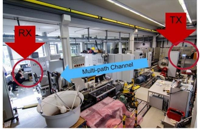
Fig. 9. Non-LoS scenario: Schematic of the machine hall setup
