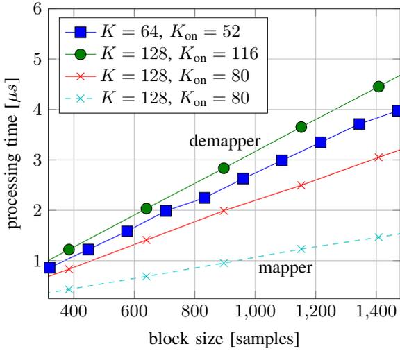
Fig. 3. Latency measurement for resource mapping [dashed] and demapping [solid] with different numbers of subcarriers  $K$  and active subcarriers  $K_{\text{on}}$ .
