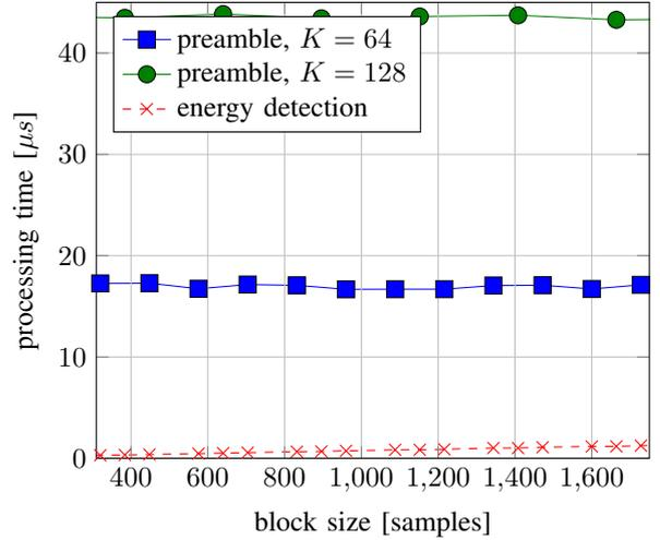
Fig. 6. Latency measurement for synchronization stages with different number of subcarriers  $K$ .
