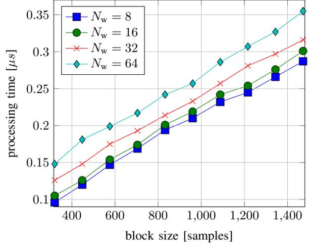
Fig. 5. Latency measurement for CP addition and windowing with different window roll-off sizes.
