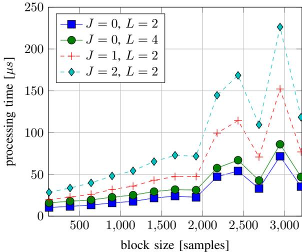
Fig. 7. Latency measurement for GFDM demodulation with increasing block size and different number of IC iterations with  $K = 128$ ,  $K_{\text{on}} = 80$
