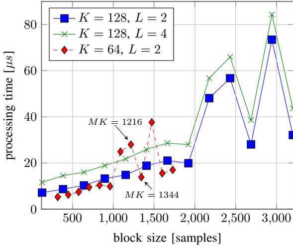
Fig. 4. Latency measurement for GFDM modulation with increasing block size.
