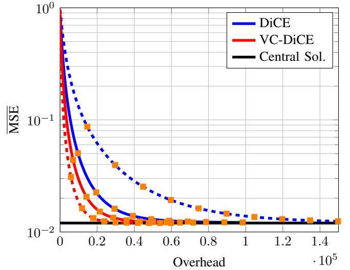
Fig. 3.  $\overline{\text{MSE}}$  vs. number of total communication overhead measured in vector elements,  $J = U = 5, N_T = 1, N_R = 2$ , the network is randomly connected (—) and fully connected (···), each marker represents an increment of 50 iterations
