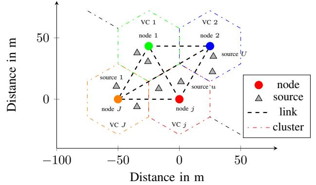
Fig. 2. A network of  $J$  nodes with the virtual cluster for each. All nodes cooperate through inter-node links to detect the common messages from  $U$  sources located in different virtual clusters.
