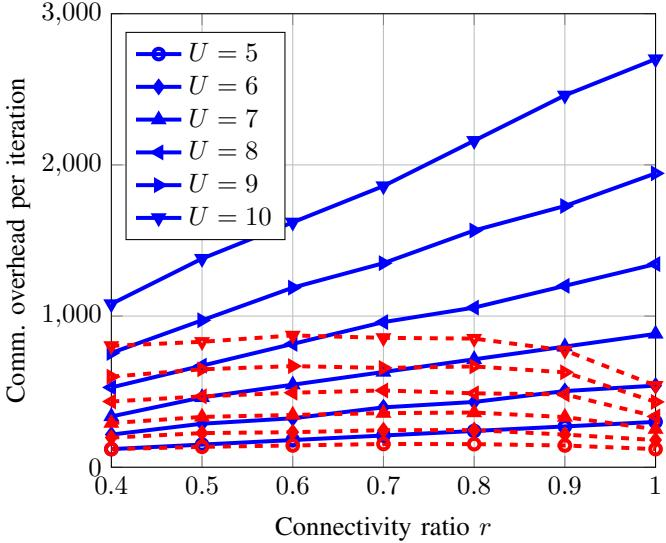
Fig. 4. Number of all N2N communication overhead per iteration measured in vector elements generated by the VC-DiCE algorithm (---) and the DiCE algorithm (—) for a network with various connectivity ratio  $r$ ,  $J = U = 5, \dots, 10$ ,  $N_T = 1$ ,  $N_R = 2$ .
