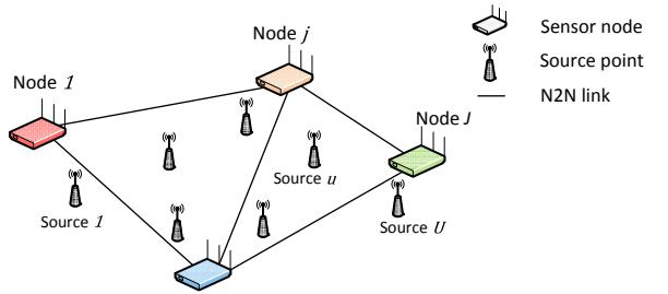
Fig. 1. A sensor network with  $J$  nodes receiving and detecting the common messages from  $U$  sources in a cooperative way.
