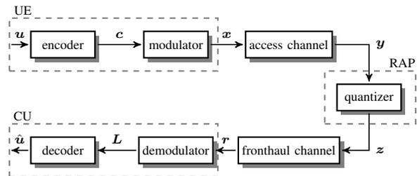
Fig. 1. The system model for the uplink of Cloud-RAN for a single UE
