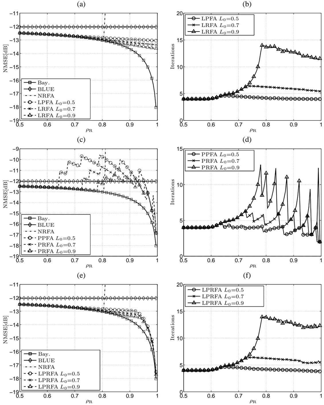
**Fig. 3.** NMSE vs.  $\rho_R$  of LRFA (a) PRFA (c) and LPRFA (e) for  $(N = 8 \times M = 8)$  system with  $K = 8$  pilot symbols at 12 dB SNR. Corresponding mean number of required iterations until convergence vs.  $\rho_R$  for LRFA (b) PRFA (d) and LPRFA (f).
