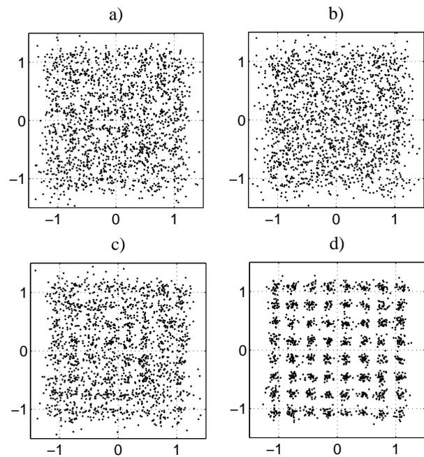
Fig. 12: Signal constellations: a) receive signal 1, b) receive signal 2, c) MRC of receive signals 1 and 2, d) MRC of receive signals 1 to 4
