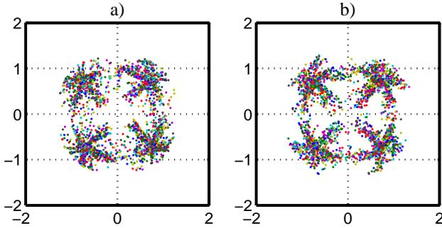
Fig. 9: QPSK signal constellations at the STBC decoder output: a) simulated signal, b) measured signal
