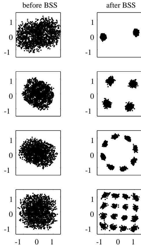
Fig. 15: 4x4 signal constellations before and after BSS
