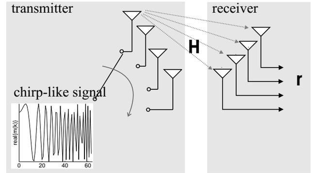
Fig. 6: Multiplexing for channel measurement
