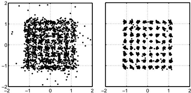
Fig. 10: Impact of a DC offset (7 dB): signal constellation diagram (uncorrected/corrected)
