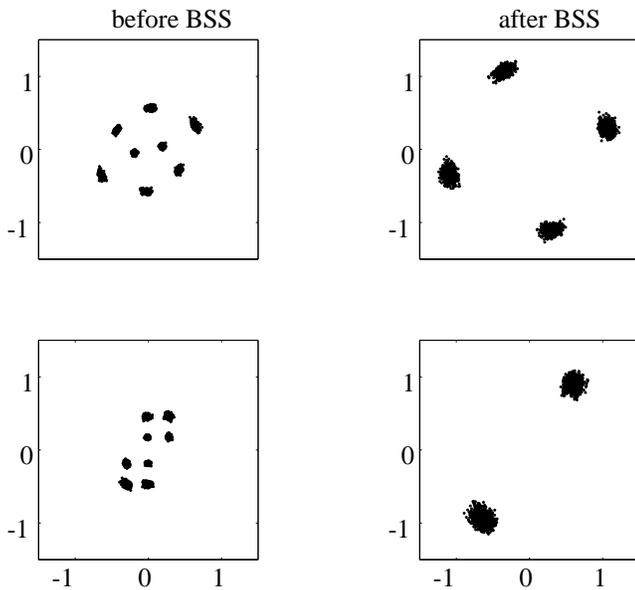
Fig. 14: 2x2 signal constellations before and after BSS
