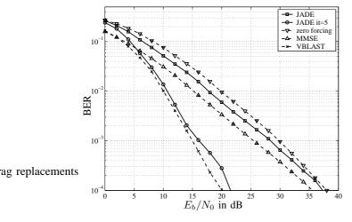
Fig. 6. BER of JADE with iterative VBLAST detection
