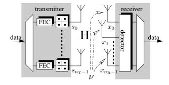
Fig. 7. transmission system with channel coding
