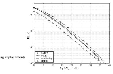
Fig. 4. BER error rates of the source separation approaches using HOS
