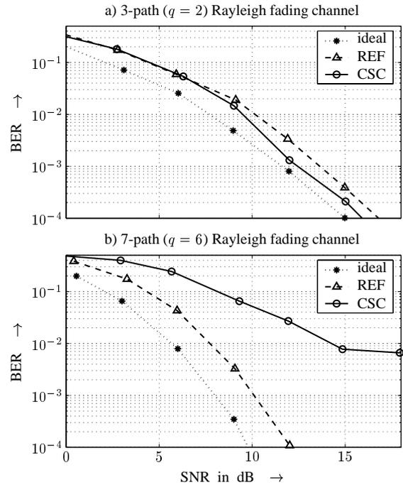
Fig. 5. BERs after chan. decod. for a HIPERLAN/2 system with  $J = 4$  (QPSK),  $N = 52$ ,  $N_{cp} = 16$  and an “ideal”, nonblind (“REF”), and blind (“CSC”) estimation of a 3-path (a) and a 7-path Rayleigh fading channel (b).
