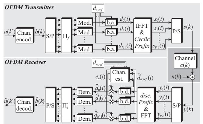
Fig. 1. Conventional OFDM system with Cyclic Prefix
