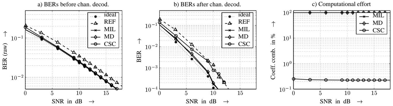
Fig. 4. BERs before (a) and after channel decoding (b) for an “ideal”, nonblind (“REF”), and blind (“MIL”, “MD”, “CSC”) channel estimation with  $J = 2$  (BPSK),  $N = 14$ ,  $N_{cp} = 6$ , and  $q = 3$ . Subplot (c) shows the computational effort of the three blind channel estimators.
