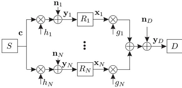
Fig. 1. Block diagram of a relay network with  $N$  parallel relays
