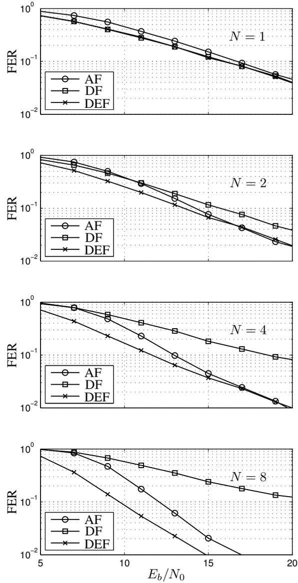
Fig. 5. Frame Error Rate vs.  $E_b/N_0$  for different relay protocols with 1, 2, 4 and 8 relays, both hops Rayleigh fading,  $[5\ 7]_8$  convolutional code
