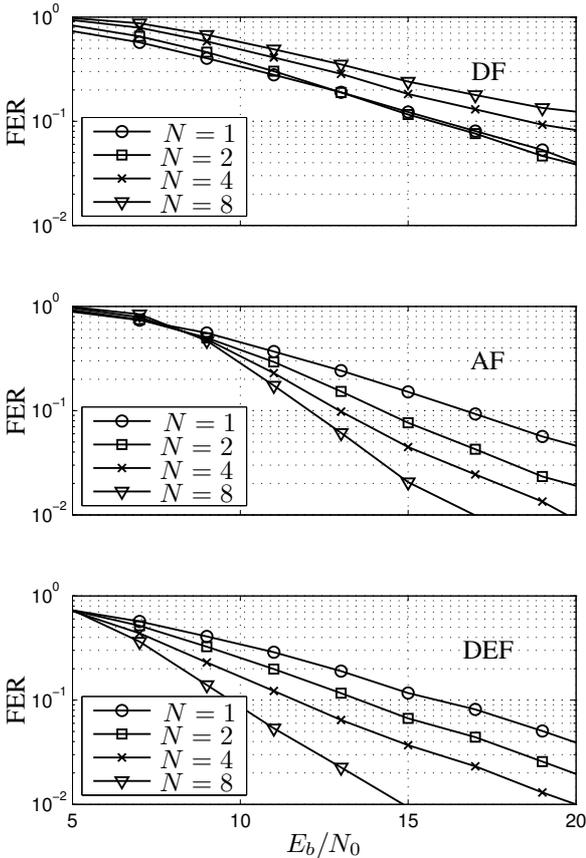
Fig. 4. Frame Error Rate vs.  $E_b/N_0$  with 1, 2, 4 and 8 relays for different relay protocols, both hops flat Rayleigh fading,  $[5\ 7]_8$  convolutional code
