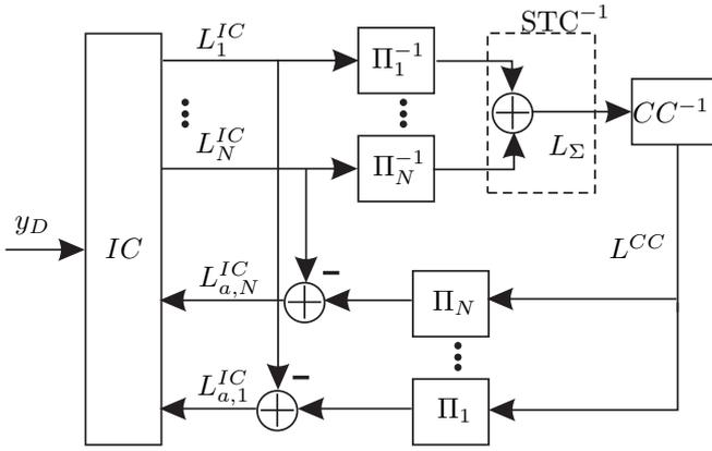
Fig. 3. Block diagram of the IDM-STC detector at the destination
