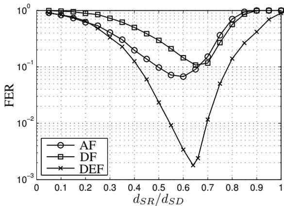
Fig. 6. Frame Error Rate vs. distance between Source and Relays for different relay protocols with 4 relays, first hop AWGN, second hop Rayleigh fading,  $[5\ 7]_8$  convolutional code
