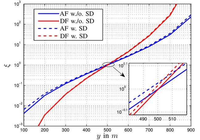
Fig. 8. Power proportion  $\xi$  of uncoded AF and DF for  $P_e^{\text{tar}} = 10^{-4}$  with  $\alpha = 4$  in a one-dimensional region ( $x = 0$ ).
