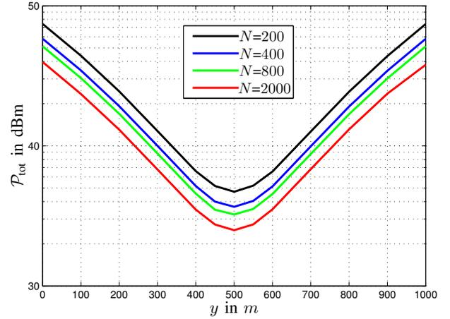
Fig. 7.  $\mathcal{P}_{\text{tot}}$  of coded DF without SD link for  $P_e^{\text{tar}} = 10^{-4}$  with  $\alpha = 4$  in a one-dimensional region ( $x = 0$ ). LDPC codes of rate  $R_C = 0.5$  and codeword length  $N = 200, 400, 800$  and 2000 with 16-QAM are used.
