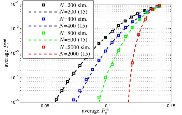
Fig. 2. Average input-output BER characteristic for an LDPC decoder of  $R_C = 0.5$  and codeword length  $N = 200, 400, 800$  and 2000 in an AWGN channel with 16-QAM modulation.
