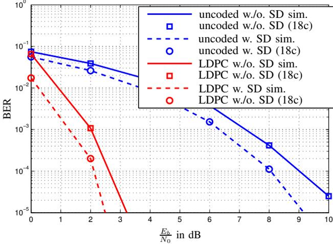
Fig. 3. BER obtained by simulation and by approximation (18c) for uncoded and coded DF with and without SD link. R joins the line between S and D with  $\frac{d_{\text{SR}}}{d_{\text{SD}}} = 0.3$ .
