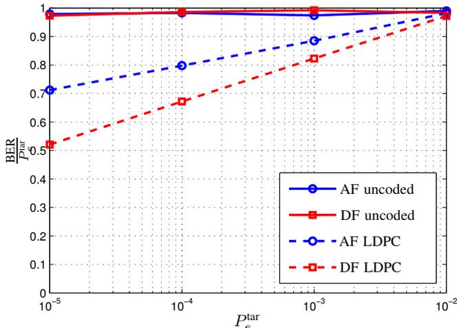
Fig. 9. Comparison of BERs achieved by simulations and the corresponding  $P_e^{\text{tar}} = 10^{-2}, 10^{-3}, 10^{-4}$  and  $10^{-5}$  with  $\alpha = 4$ ,  $x = 0$  and  $y = 500$ .
