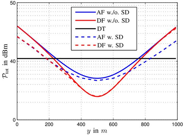
Fig. 6.  $\mathcal{P}_{\text{tot}}$  of coded AF and DF with SD link and without SD link for  $P_e^{\text{tar}} = 10^{-4}$  with  $\alpha = 4$  in a one-dimensional region ( $x = 0$ ). An LDPC code of rate  $R_C = 0.5$  and codeword length  $N = 2000$  with 16-QAM is used.
