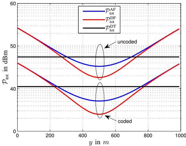
Fig. 4.  $\mathcal{P}_{\text{tot}}$  of AF and DF without SD link for  $P_e^{\text{tar}} = 10^{-4}$  with  $\alpha = 4$  in a one-dimensional region ( $x = 0$ ).
