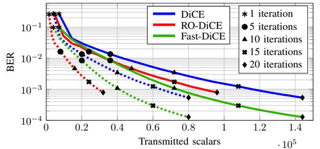
Fig. 2. BER versus communication overhead for P2P (—) and P2MP (····) inter-node links for fixed  $E_b/N_0 = 10$  dB.
