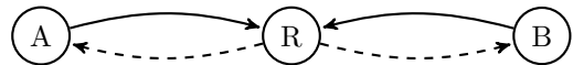
Fig. 1: A TWRC with MAC phase (solid lines) and BC phase (dashed lines).
