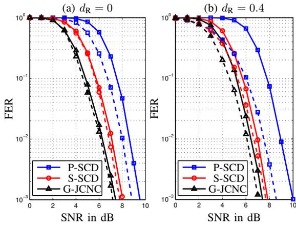
Fig. 4. FER performance versus SNR for both traditional (-) and modified (- -) adaptive schemes using P-SCD, S-SCD and G-JCNC at the relays, (a) is for  $d_R = 0$  and (b) is for  $d_R = 0.4$ .
