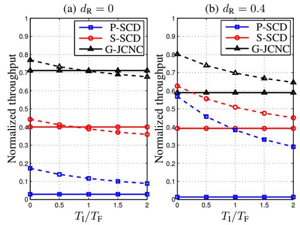
Fig. 6. Normalized throughput versus  $T_I/T_F$  for both traditional (-) and modified (- -) adaptive schemes using P-SCD, S-SCD and G-JCNC at the relays with SNR = 4dB, (a) is for  $d_R = 0$  and (b) is for  $d_R = 0.4$ .
