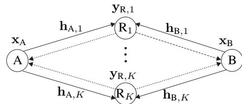
Fig. 1. A two-way relaying network consisting of a MA phase (solid lines) and a BC phase (dashed lines) where two sources A and B exchange messages with each other via  $K$  distributed relays  $R_k$ ,  $k = 1, \dots, K$ .
