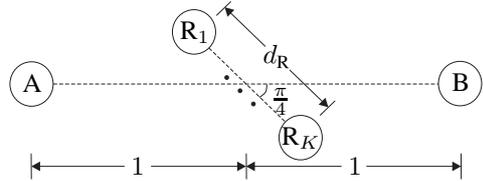
Fig. 3. A two-way relaying network with  $K$  linearly positioned relays. Equal distance is assumed between neighboring relays. The two lines connecting the sources and the relays respectively form an angle of  $\pi/4$ .
