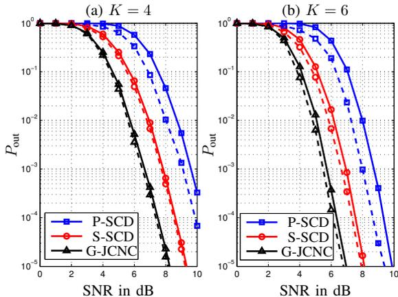
Fig. 2. Outage probability  $P_{\text{out}}$  versus SNR for both traditional (-) and modified (- -) adaptive schemes using P-SCD, S-SCD and G-JCNC at the relays. A symmetric network is considered with (a)  $K = 4$  relays and (b)  $K = 6$  relays. The rate of the BC phase is set to  $R = 0.5$ .
