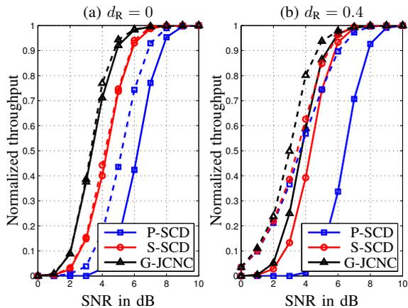
Fig. 5. Normalized throughput versus SNR for both traditional (-) and modified (- -) adaptive schemes using P-SCD, S-SCD and G-JCNC at the relays with  $T_I = 0$ , (a) is for  $d_R = 0$  and (b) is for  $d_R = 0.4$ .
