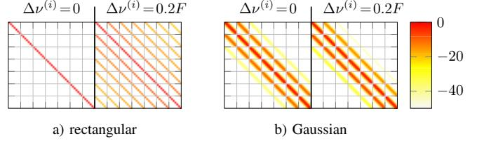
Fig. 2. Matrices  $\mathbf{V}_i$  for a) rectangular waveform and b) Gaussian waveform. Flat fading channel with and without influence of additional CFO.
