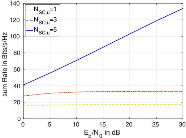
Fig. 4. Sum rate w.r.t.  $\frac{E_b}{N_0}$  for proposed algorithm using  $K = 30$  iterations, considering no cooperation, partial cooperation and full cooperation
