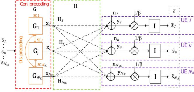
Fig. 1. Diagram of signal processing in central/distributed precoding
