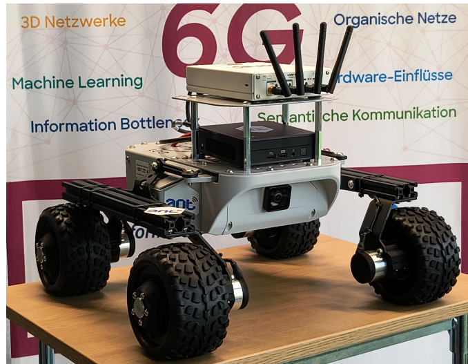
Fig. 2. LeoRover with Intel NUC and B210 SDR
