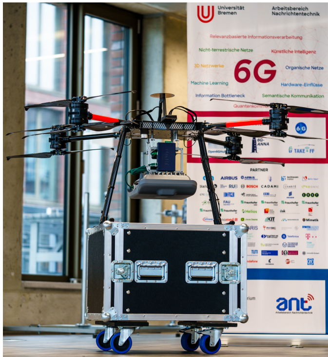
Fig. 3. MK-U25 drone with 5G outdoor BS and 5G core
