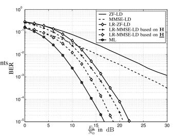
Fig. 3. Bit Error Rate of a system with  $n_T = 4$  and  $n_R = 4$  antennas, 4-QAM symbols, ZF (continuous lines) and MMSE (dashed lines) linear detection.
