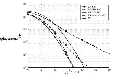
Fig. 4. Bit Error Rate of a system with  $n_T = 4$  and  $n_R = 4$  antennas, 4-QAM symbols, ZF (continuous lines) and MMSE (dashed lines) optimally sorted SIC detection.
