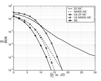
Fig. 5. Bit Error Rate of a system with  $n_T = 6$  and  $n_R = 6$  antennas, 4-QAM symbols, ZF (continuous lines) and MMSE (dashed lines) optimally sorted SIC detection.
