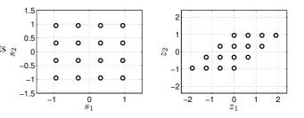
Fig. 2. Original 16-QAM symbols  $\mathbf{s} \in \mathcal{A}^2$  with  $\mathcal{A} = \{\pm \frac{1}{2}a, \pm \frac{3}{2}a\}$  (left) and transformed symbols  $\mathbf{z} \in \mathbf{T}^{-1}\mathcal{A}^2$  (right).
