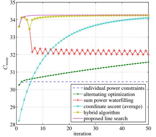
Fig. 6. Convergence behavior of sum rate maximization algorithms
