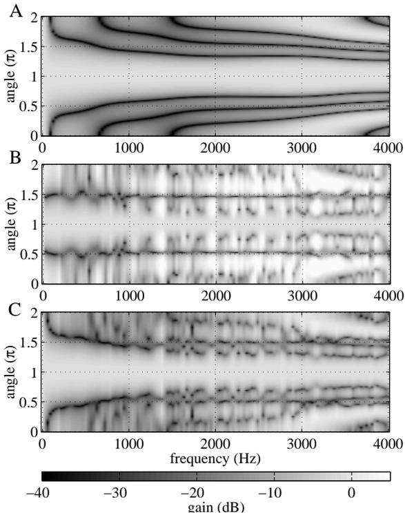
Figure 3: Beam pattern of a superdirective beamformer (A), an optimally designed beamformer (B), and linear interpolation between them with  $\delta = 0.75$  (C).
