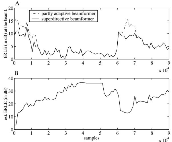
Figure 4: ERLE at the beamformer after a preceding multi-channel AEC (A). The RIRs are exchanged at 60,000 samples. The adaptive beamformer is switched on, when the estimated ERLE (B) falls below 20dB.
