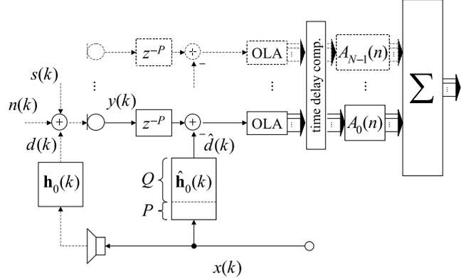
Figure 1: Signal model of a combined structure with a multi-channel AEC-unit in front of a beamformer.
