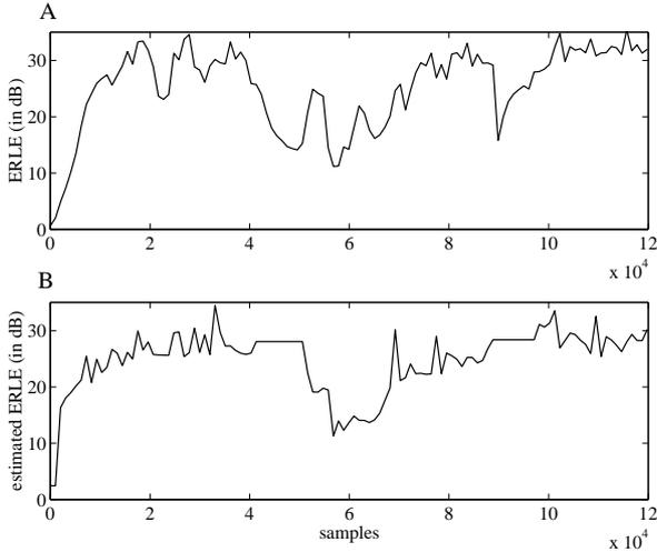
Figure 2: ERLE (A) and estimated ERLE (B) measured at an AEC. There is a sudden modification of the RIR at 55,000 samples. A near-end speaker is active between sample 80,000 and 100,000. The far-end speaker pauses at 40,000 and 90,000 samples.
