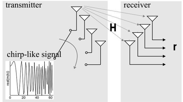
Fig. 6: Multiplexing for channel measurement
