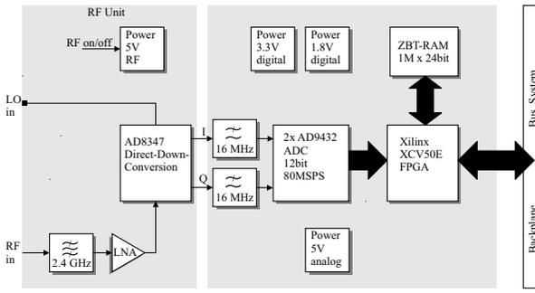
Fig. 3: Receiver module
