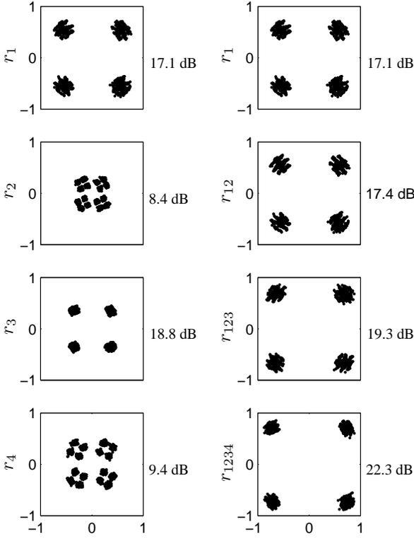
Fig. 8: Combining gain with estimated SNR
