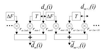
**Fig. 6:** Transmission model of the simple two-dimensional channel impulse response of Equation 7.
