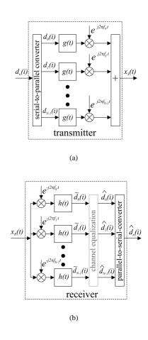
Fig. 1: Block diagram of a multicarrier system, (a): transmitter, (b): receiver
