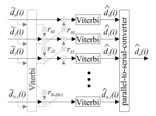
**Fig. 4:** Pseudo two-dimensional equalization structure; in black the time-direction equalization, in grey the frequency-direction components.
