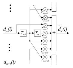
Fig. 2: Two-dimensional transmission model for MCSIS with  $r_{nmi} = r_{n,m}(iT)$
