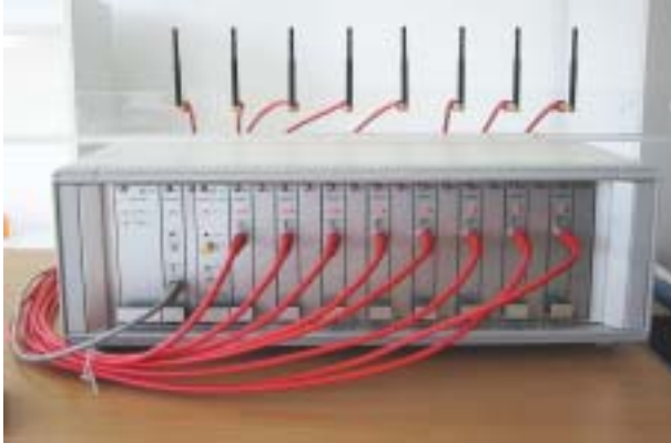
Fig. 2. The Multiple Antenna Receiver for ISM-Band Transmission. Currently, the receiver and transmitter are equipped with 8 modules.
