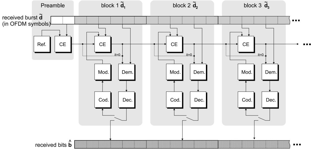
Fig. 1. Iterative channel estimation for a received burst
