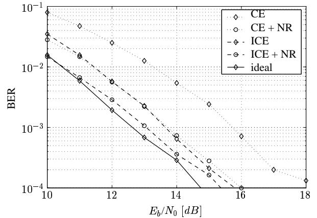
Fig. 2. Simulation results: BER Hiperlan/2 conditions
