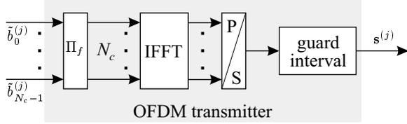
**Figure 2:** Typical structure of an OFDM-CDMA transmitter
