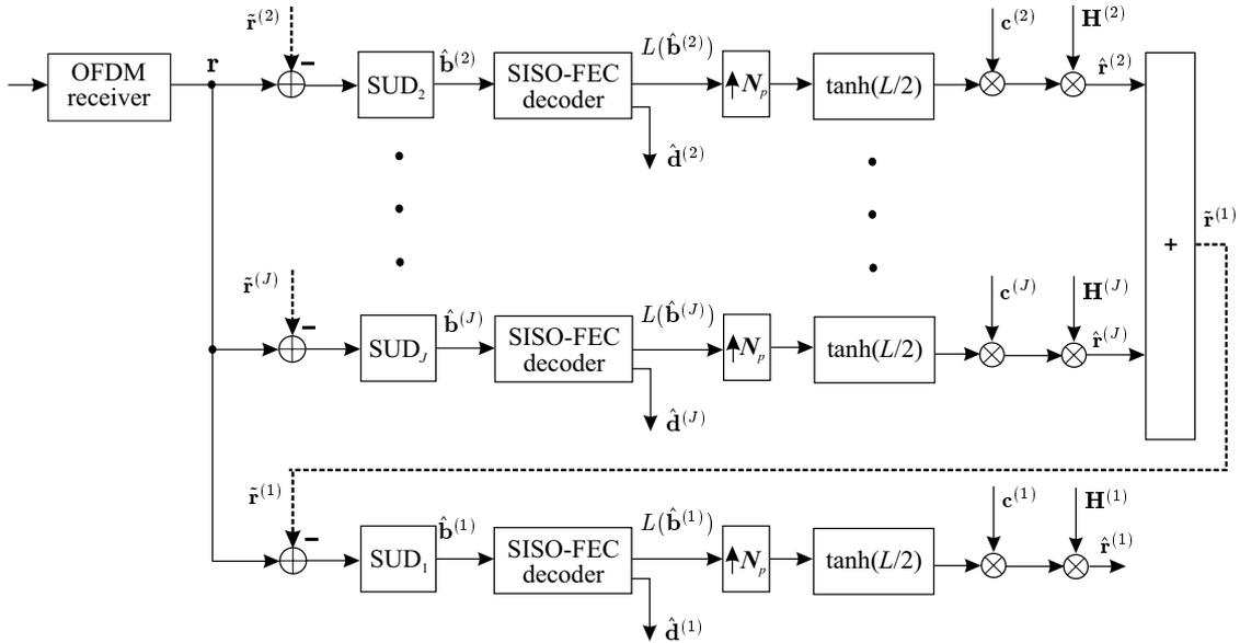
Figure 7: Principle structure of the parallel interference cancellation scheme
