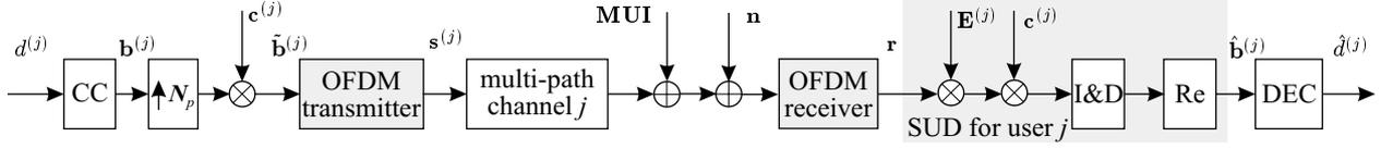
**Figure 1:** Typical structure of an OFDM-CDMA system with single-user detection
