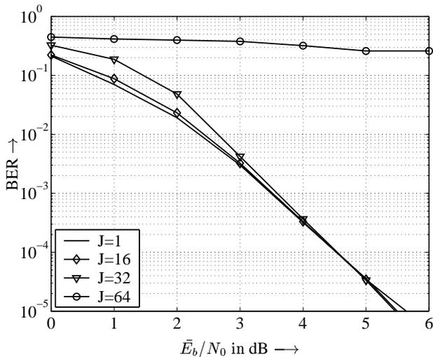
Figure 8: Performance of PIC with 3 iterations for different number of users
