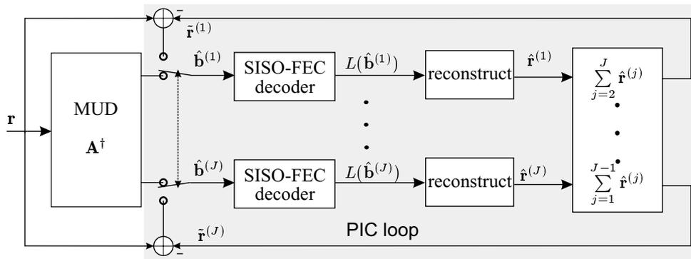
Figure 9: Combination of linear MUD and parallel interference cancellation
