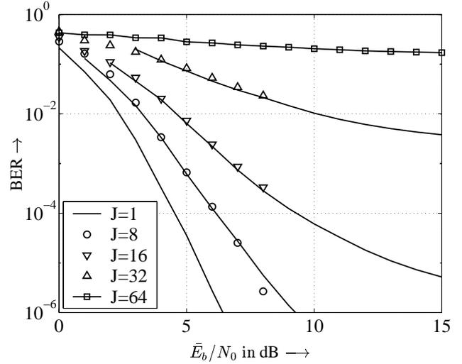
**Figure 4:** Simulation results for convolutional code with  $R_c = 1/2$ , different number of active users
