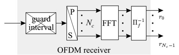
**Figure 3:** Typical structure of an OFDM-CDMA receiver
