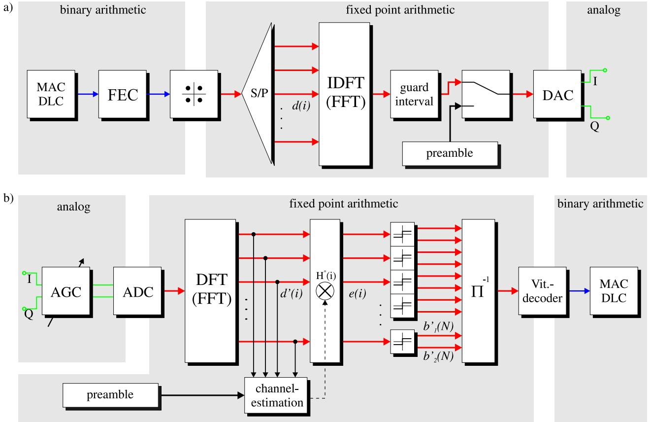
**Figure 1:** a) OFDM transmitter with channel coding and DAC; b) OFDM receiver with ADC and channel decoding
