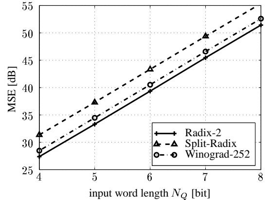
Figure 4: internal quantization effects
