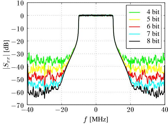
**Figure 9:** power density spectrum of transmitter output signal
