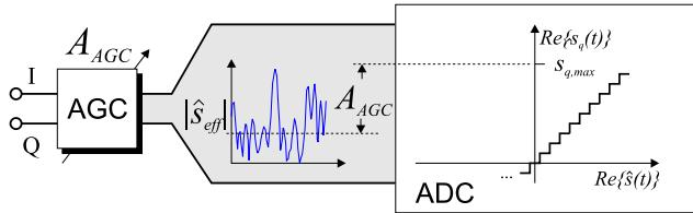
**Figure 5:** ADC input level  $A_{AGC}$
