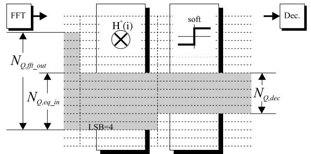
**Figure 7:** data word length while equalizing
