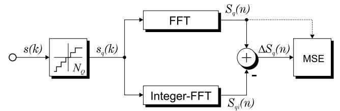
Figure 3: simulation of internal quantization effects
