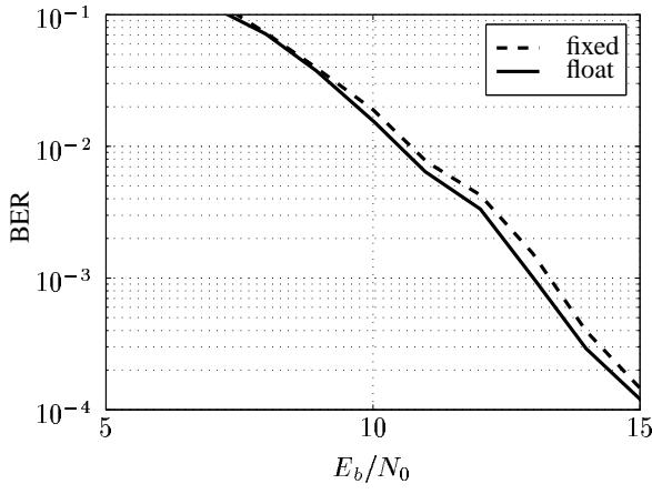
**Figure 8:** system performance of fixed point model and floating point model
