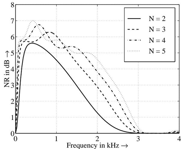
Figure 5: Additional noise reduction performance of SDBs ( $d = 5\text{ cm}$ ) for different numbers of sensors  $N$  (endfire)
