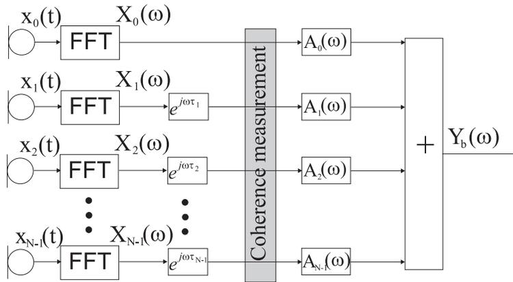
Figure 1: Block diagram of a superdirective beamformer in a frequency domain implementation, including measurepoints of coherence
