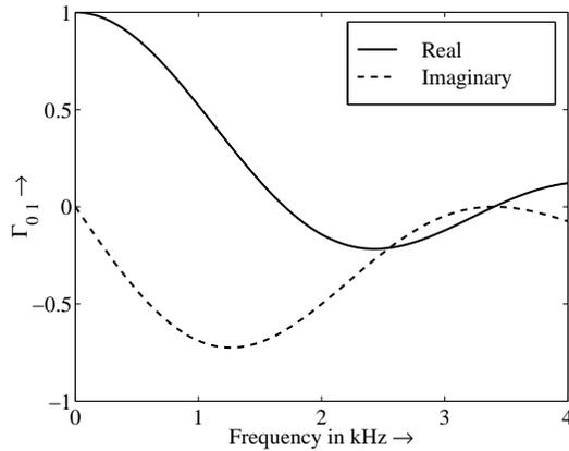
Figure 3: Complex coherence function in a diffuse noise field after endfire steering ( $d = 5\text{cm}$ )
