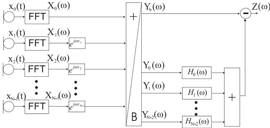
Figure 2: Block diagram of a GSC-like superdirective beamformer in a frequency domain implementation
