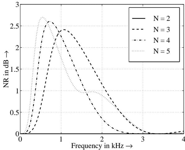
Figure 4: Additional noise reduction performance of SDBs ( $d = 5\text{ cm}$ ) for different numbers of sensors  $N$  (broadside) (note that there is no additional noise reduction for  $N = 2$ )
