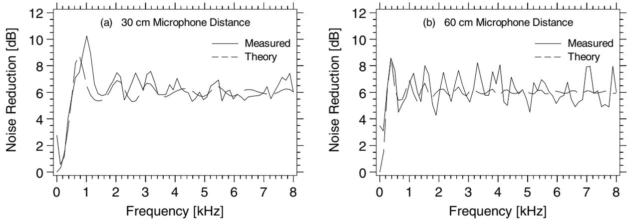
**Fig 6** Noise reduction of the non-adaptive beamformer as a function of frequency (eq. 22)
