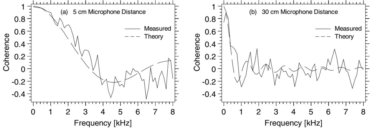
Fig. 5. Real part of the complex coherence function (eq. 3 and 4) measured in an office room.
