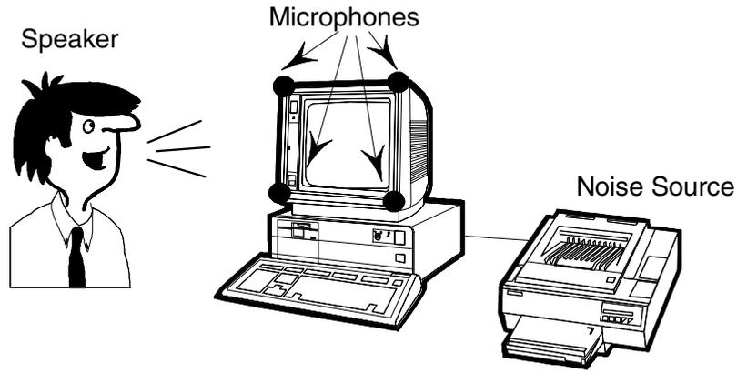
Fig. 1 Hardware configuration of the adaptive array
