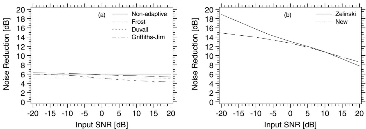
Fig. 3 Noise reduction of different algorithms as function of input SNR in an office room.
