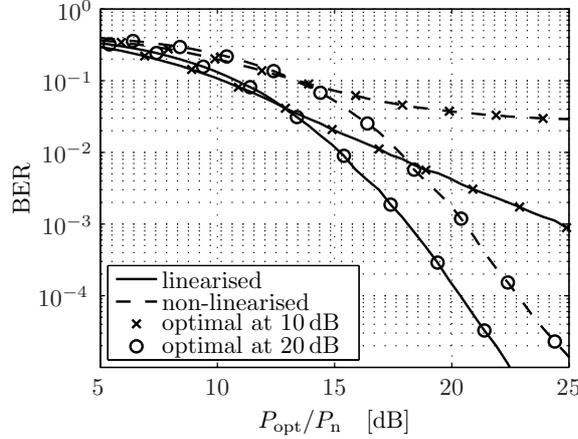
Figure 3. Bit error performance of a linearised IM/DD OFDM system for the optimal parameters  $b_{\text{pre}}, m_{\text{pre}}\sigma_x$  in two operating points in dependence on the power ratio  $P_{\text{opt}}/P_n$  and bit error performance of the non-linearised system as a reference
