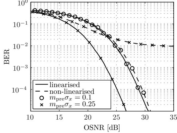
Figure 4. Bit error performance of a linearised IM/DD OFDM system in comparison to a non-linearised system
