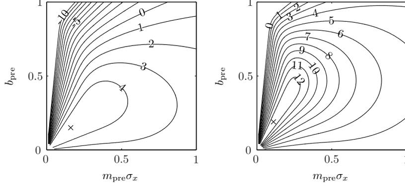
Figure 2. Signal-to-interference-and-noise ratio in dB for noise powers  $P_{\text{opt}}/P_n = 10$  dB (left), 20 dB (right) and varying parameters  $b_{\text{pre}}, m_{\text{pre}}\sigma_x$
