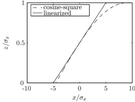
Figure 5. Comparison of characteristics of linearised and non-linearised system for  $b_{\text{pre}} = 0.5$  and  $m_{\text{pre}}\sigma_x = 0.1$
