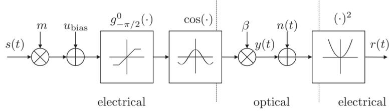
Figure 1. Block diagram of the physical components of the transmission system
