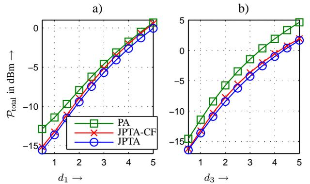
Figure 5: Impact of distance on  $\mathcal{P}_{\text{total}}$  in dBm for only power optimized ( $\alpha_k = 1/K, \forall k$ ) and joint power and time allocation for adaptive scheme. a)  $d_1$  varies from 0.5km to 5km; b)  $d_3$  varies from 0.5km to 5km.
