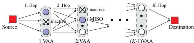
Figure 1: Topology of adaptive distributed MIMO multi-hop relaying systems.
