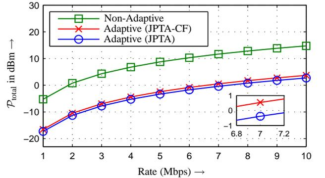
Figure 2:  $\mathcal{P}_{\text{total}}$  in dBm for non-adaptive transmission, closed-form and optimal resource allocation solution.
