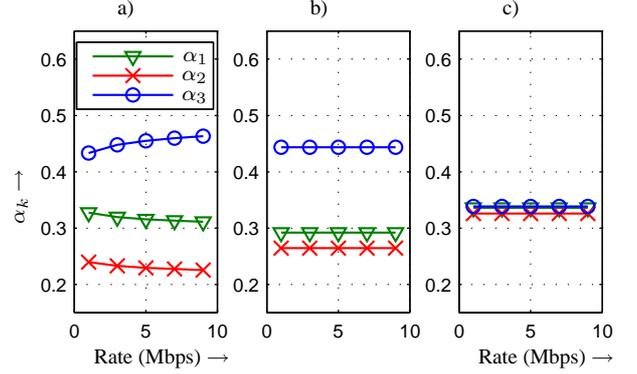
Figure 7: The time fraction  $\alpha_k$  per hop for a) *JPTA-CF*, b) *JPTA*<sub>1</sub> and c) *JPTA*<sub>2</sub>.
