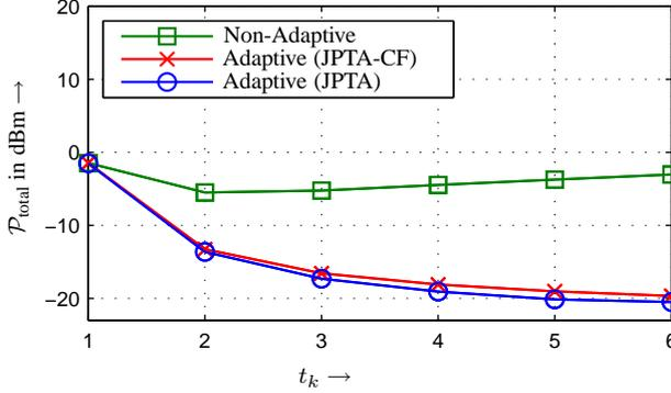
Figure 3:  $\mathcal{P}_{\text{total}}$  in dBm versus different number of nodes per VAA from 1 to 6 for non-adaptive transmission, closed-form and optimal resource allocation solution,  $R = 1\text{Mbps}$ .
